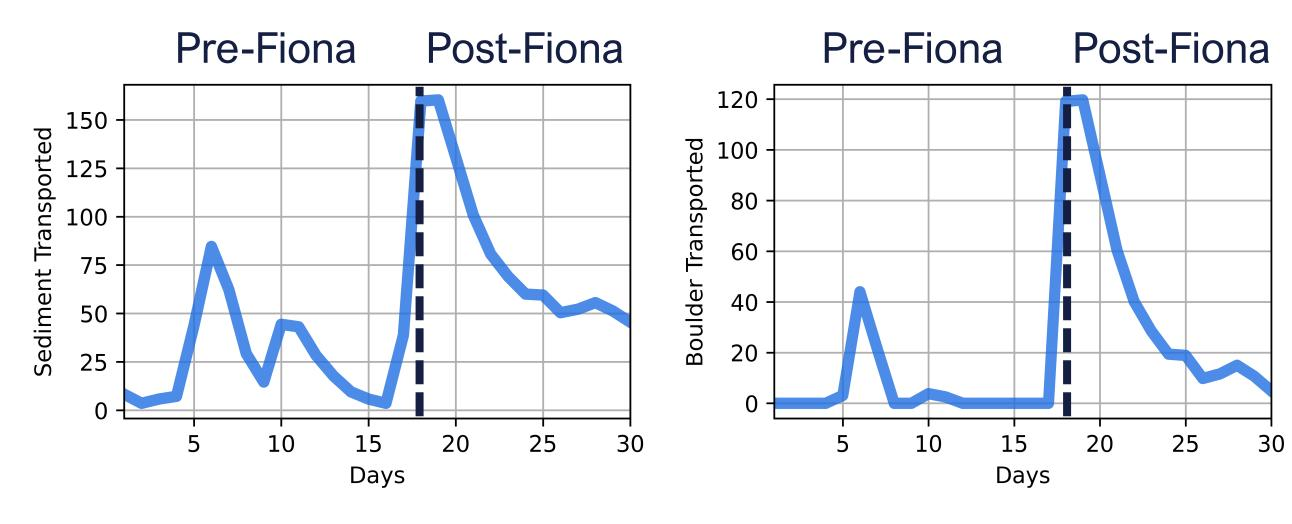
pre-Fiona sediment transported: 297, 54 boulders post-Fiona sediment transported: 872, 419 boulders
